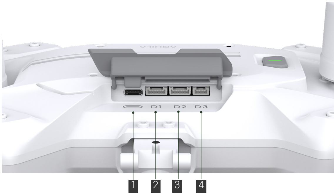
1.Expansion Board USB-C Port (Debug Port) 2.Serial Interface D1
